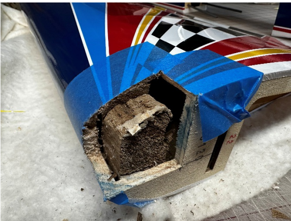
Picture 1 : Leading Edge Battery Cut Out
